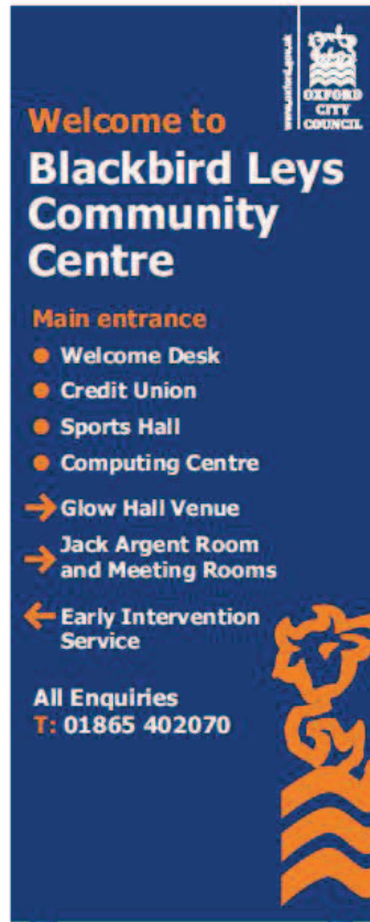
1.0 Front-facing road Internally mounted post monolith 2500mm x 1000mm; approx. 100mm returns (2950mm x 920mm is an off shelf item) 500mm of 80mm posts in ground. Powder Coated RAL 5002 vinyl graphics artwork supplied.
